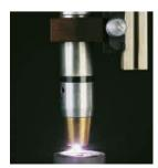
Plasma Transferred Arc (PTA) surfacing is ideal for high unit volume automated applications, such as thermal surfacing of exhaust valves. Low base metal dilution and a wide range of consumables are two of several advantages that the technique can offer.
