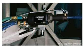
HVOF is the surfacing method of choice when extremely high-density coatings are required. The process is easily automated and very little subsequent machining is required.
